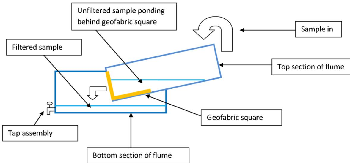
Figure 4 Schematic of flume setup
