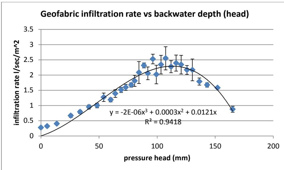
Figure 9 Infiltration rates with varying head for the clear water input condition.
