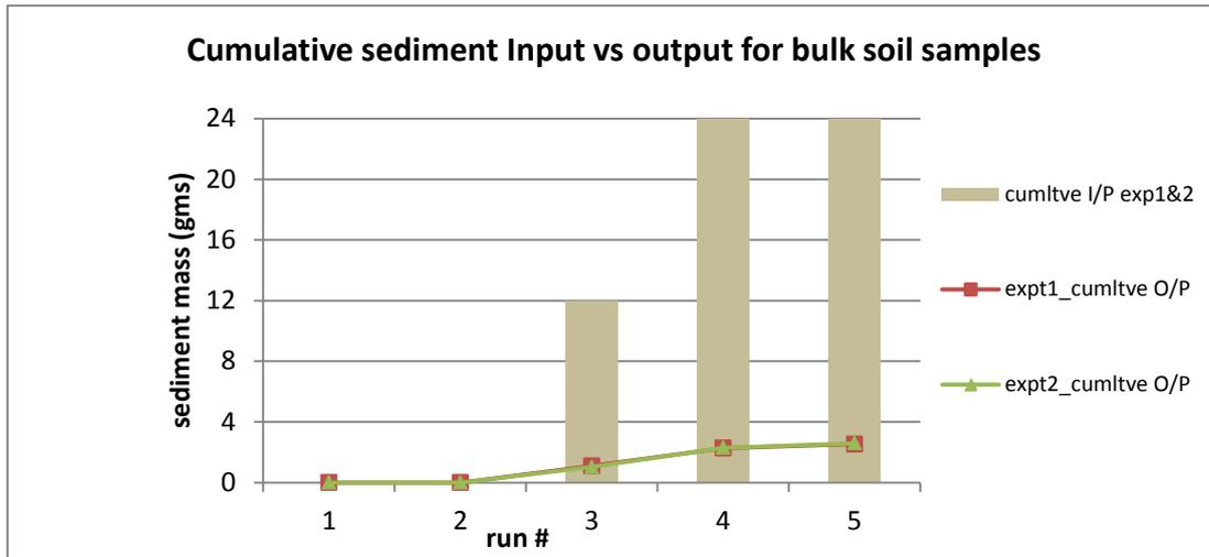
Figure 10 Results of the two experiments (multiple runs each) using the bulk sample Hodgkinson soil material. Each experiment had two initial clear water runs followed by 2 runs at 400mg/l, and a final clear water run.
