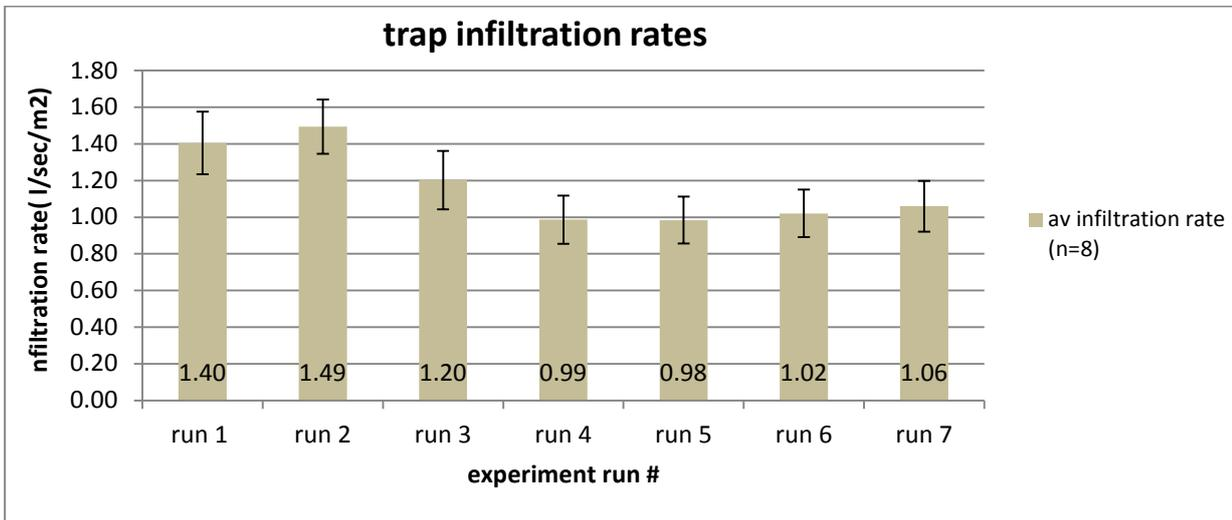
Figure 8 Average Geofabric infiltration rates (until all solution is run through) for the full set of <63 $\mu$ m Hodgkinson soil runs including the two initial clear water runs. Error bars represent one standard deviation. Note the first 2 runs are clear water runs (run 1 and 2), followed by 2 runs at 400mg/l (runs 3 and 4), then followed by a further 3 clear water runs (runs 5, 6, 7).
