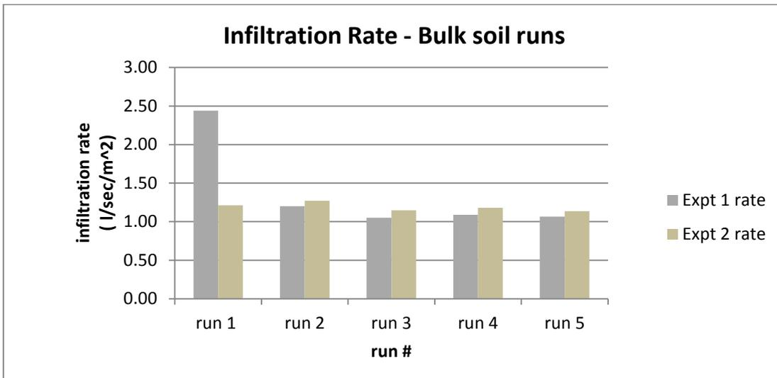
Figure 12 Infiltration rates for the geofabric with bulk soil as the input. Each experiment had two initial clear water runs followed by 2 runs at 400mg/l, and a final clear water run.
