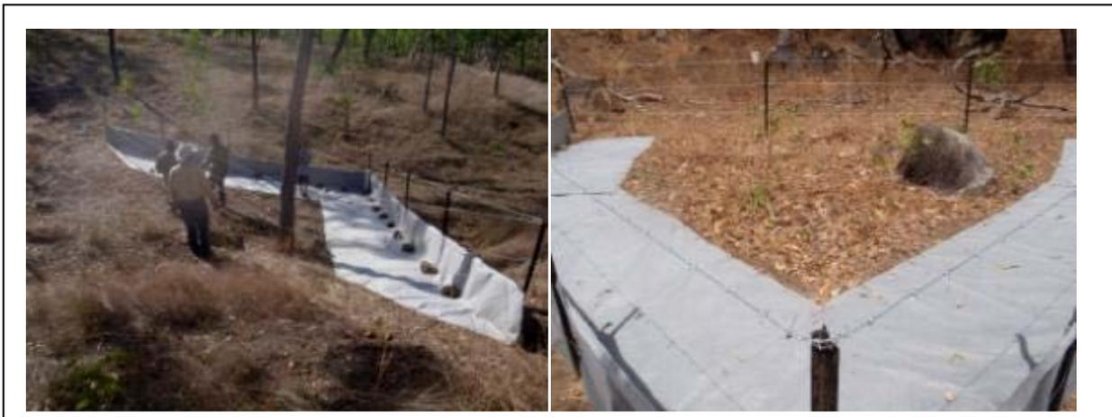
Figure 2 Examples of the two trap variants as deployed in the Normanby catchment; straight wing V shaped variant left; U shaped variant right
