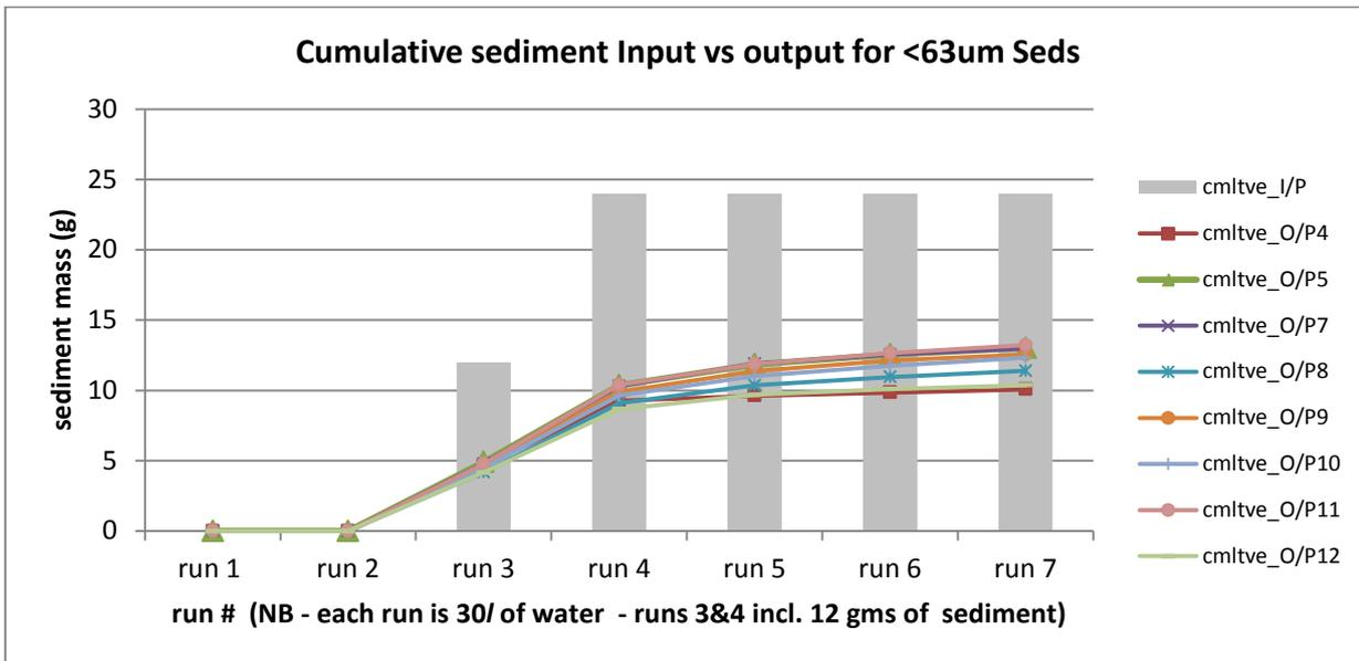
Figure 6 Results of the eight experiments run using the <63µm Hodgkinson soil material. The grey bars represent the cumulative mass of sediment input across the 7 runs – while the coloured lines represent the cumulative sediment output for the eight experiments. Note the first 2 runs are clear water runs (run 1 and 2), followed by 2 runs at 400mg/l (runs 3 and 4), then followed by a further 3 clear water runs (runs 5, 6, 7).
