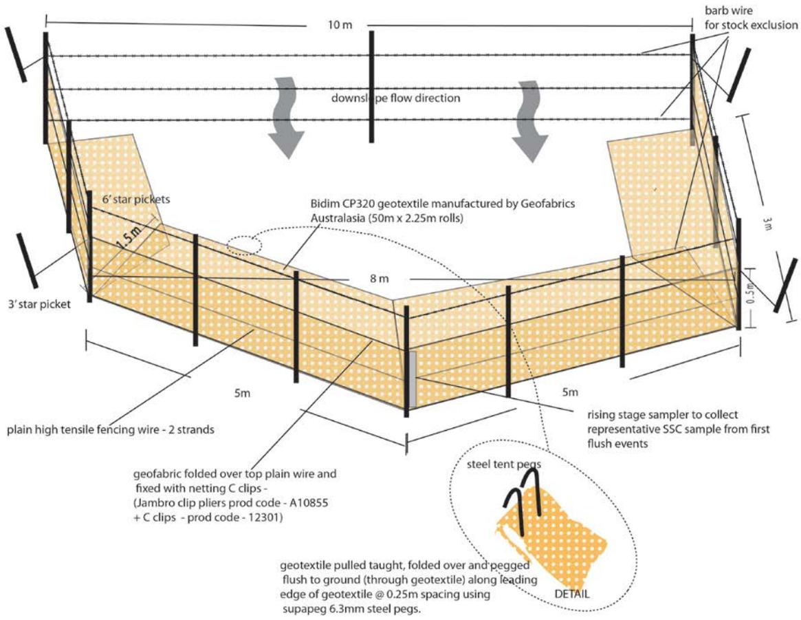
Figure 1 Design specifications for the bent wing variant of the Hillslope sediment trap
