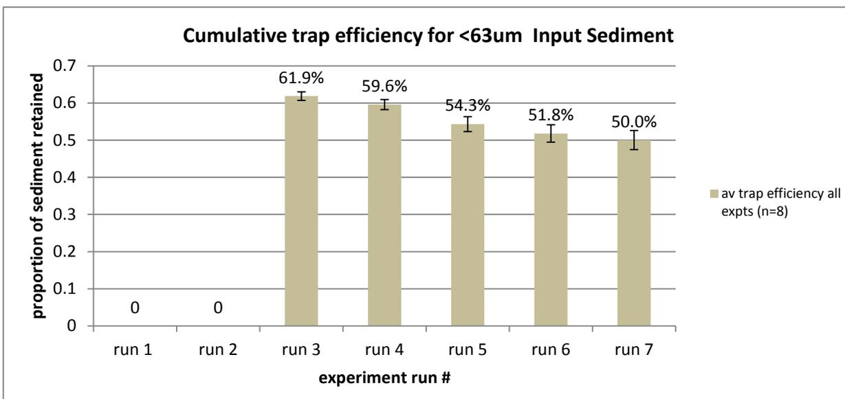
Figure 7 Cumulative trap efficiency results across the seven runs from the eight experiments replicates. Error bars represent one standard deviation. Note the first 2 runs are clear water runs (run 1 and 2), followed by 2 runs at 400mg/l (runs 3 and 4), then followed by a further 3 clear water runs (runs 5, 6, 7).
