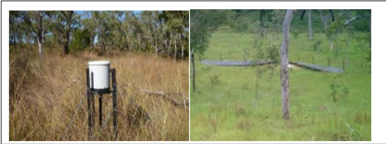
Figure 3 Examples of the tipping bucket rain gauge setup (left) and one of the traps in operation under backwater conditions during a rain event (right) in the middle of the wet season.
