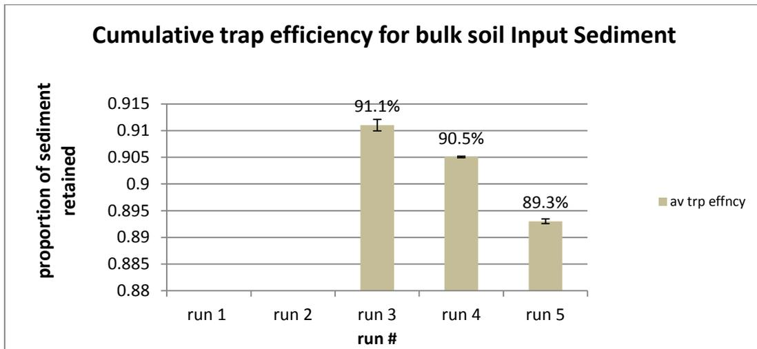
Figure 11 Cumulative trap efficiency results with bulk soil as the input load at a concentration of 400mg/l. Error bars represent one standard deviation. Each experiment had two initial clear water runs followed by 2 runs at 400mg/l, and a final clear water run.
